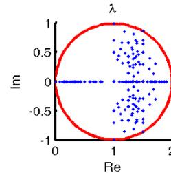
Fig. 5. Eigenvalues of all possible Laplacian matrices of topologies with 4 units
