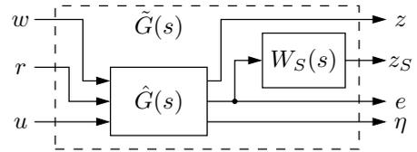
Fig. 9. Generalized plant for simultaneous local-level and formation-level robust-performance controller design
