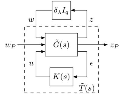
Fig. 7. Closed-loop interconnection for robust-performance controller design
