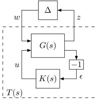
Fig. 6. Closed-loop interconnection for controller design
