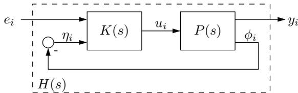
Fig. 2. Local feedback of single unit and its controller
