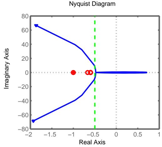
Fig. 8. Nyquist plot of  $H(s)$  and the negative inverse eigenvalue of the Laplacian corresponding to the graph in Fig. 1
