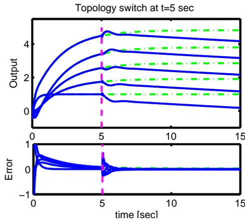
Fig. 11. Formation response to a position reference and topology change. Top figure - unit's outputs, bottom figure - unit's error signals.
