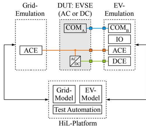
Fig. 3. Test environment for an EVSE.
