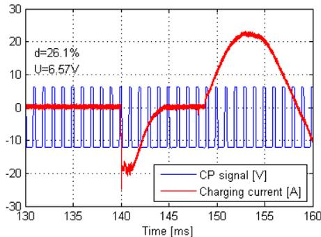
Fig. 8. Record of a CP and current at the beginning of the charging by Mode 2. Channel 1 shows the PWM communication, channel 2 the charging current.
