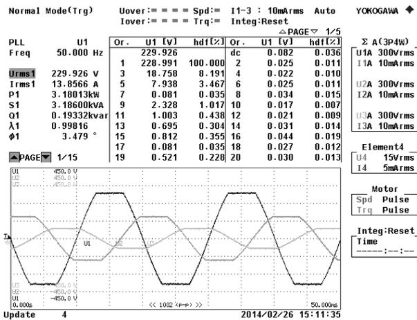
Fig. 7. Asymmetric three phase flat curve supply voltage, generated by an ACE, as specified by [17], [18]. At the top the first 20 harmonics of phase U1 are shown.
