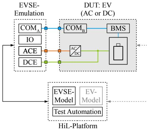
Fig. 4. Test environment for an EV.
