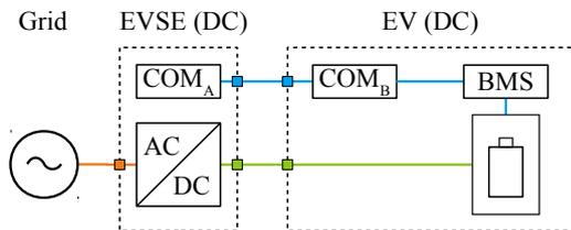
Fig. 2. Schematic diagram of DC charging in mode 4.
