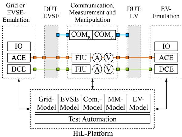
Fig. 6. Environment for testing EVSE, EV and combined EVSE and EV testing.
