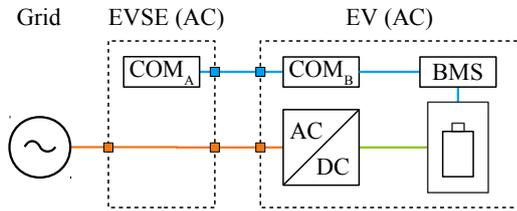
Fig. 1. Schematic diagram of on-board charging in modes 2 and 3.
