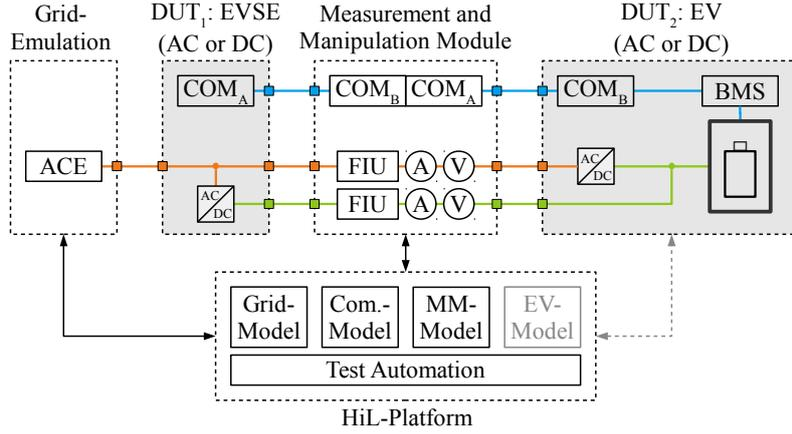
Fig. 5. Environment for combined EVSE and EV testing.
